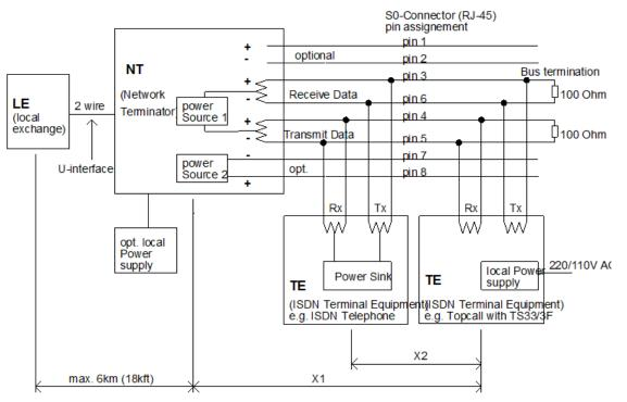
LE: Local exchange. Uses a standard 2 wire twisted pair cable for communication with NT. The twisted pair is referred to as U interface.
