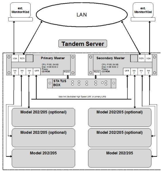
The Tandem server consists of two single servers. Both servers must be connected via two independent paths.
