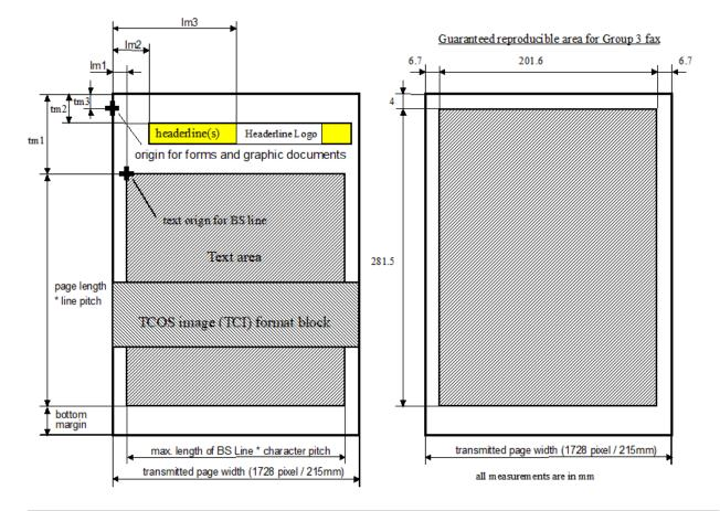
**Note** According to CCITT recommendation T.4, all information outside the guaranteed reproducible area may not be printed by the receiving fax machine. To get this reproducible area also for the ULP module, it increases all top margins by 2,7mm.
